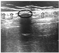
**Figure 1.** Hyperechoic lines of the pump body (arrows) and hypoechoic refill port (circled) located between the hyperechoic lines can be visualized clearly.
