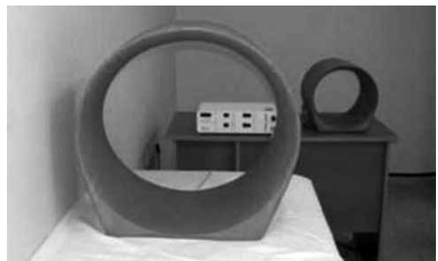
Figure 1. Power supply and solenoids of pulsed electromagnetic field therapy.
