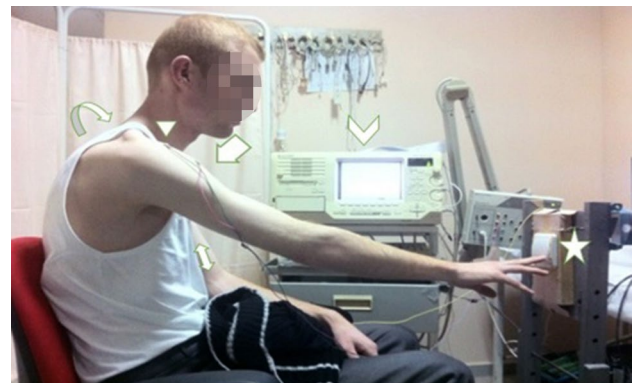
Figure 2. Experimental setup for the measurement of reaction time (arrow: active recording surface electrode placed on the anterior portion of deltoid muscle of the dominant upper extremity, triangle: reference electrode placed on the acromion of the dominant upper extremity, star: button located on the vertical platform, curved arrow: non-dominant shoulder where stimulation was performed with the surface electrode, double-headed arrow: non-dominant upper extremity, chevron arrow: stimulating [electromyography] device).
